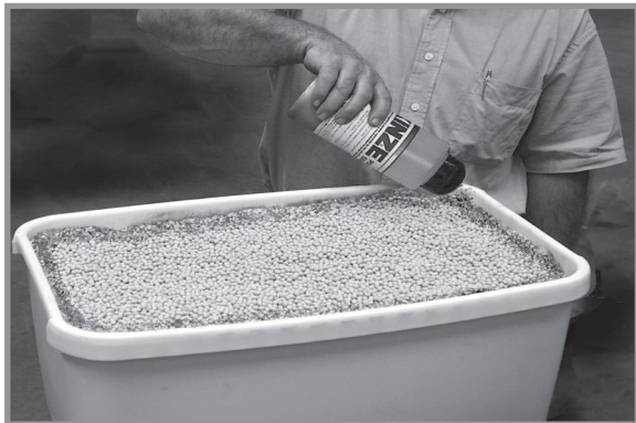
Adding graphite to conventional hopper
