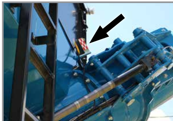
Flow Gate Position Indicator
