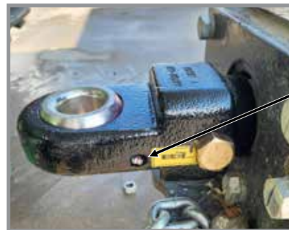
Swivel Hitch (Qty. 1) 2024 Production and On
