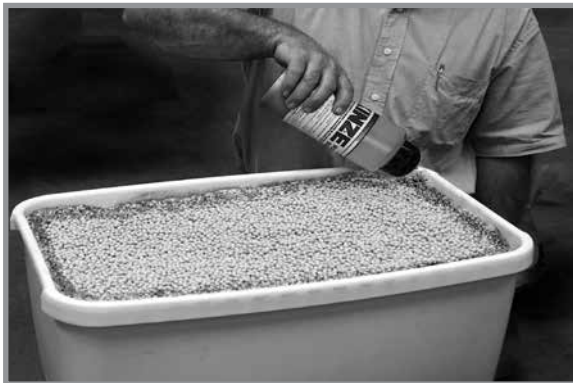
Adding graphite to conventional hopper
