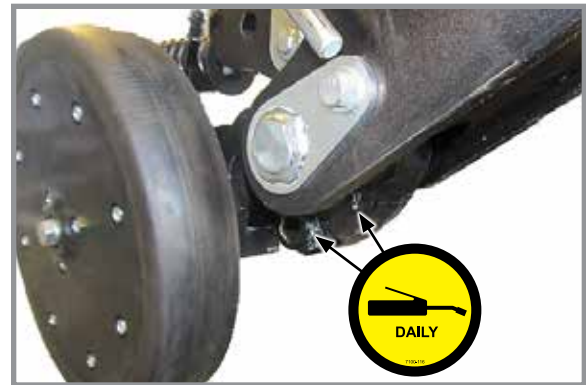
Grease to purge - 2 fittings
