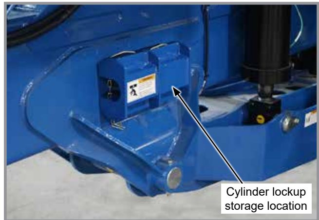
Cylinder lockup storage location
