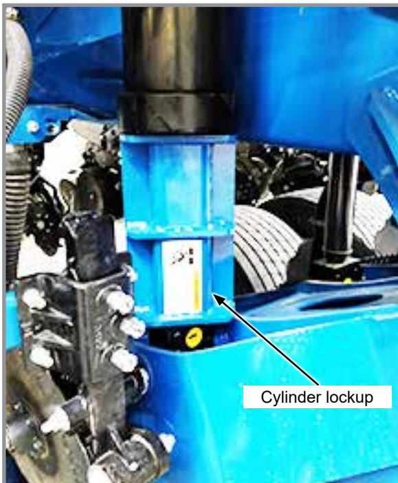
Transport axle cylinder lockup installed
