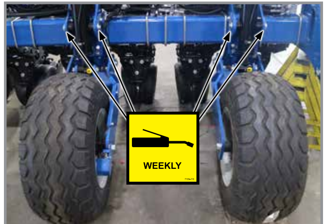
5. Lift Cylinders, 12 per machine 3 fittings per cylinder
