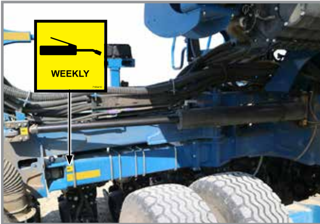
8. Stub Wing Roller, 2 per machine 1 fitting per roller
