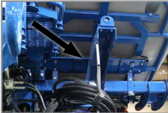
Cleanout Chute Storage Location
