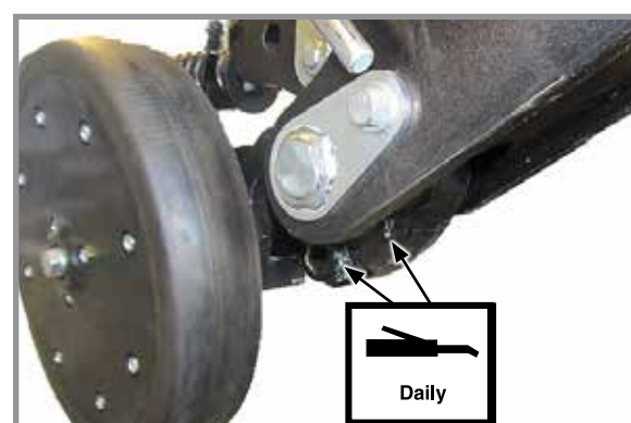
Grease to purge - 2 fittings
