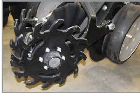
Coulter Mounted Residue Wheels
