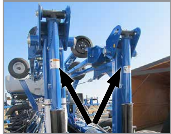
Row Marker Safety Lockup Installed
