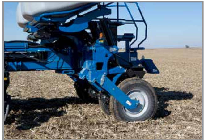
Flip Axle in Field Turnaround Position
