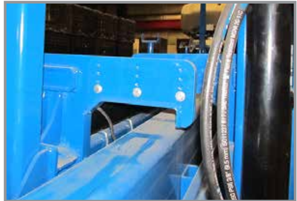
Hitch Release from Wing Hook
