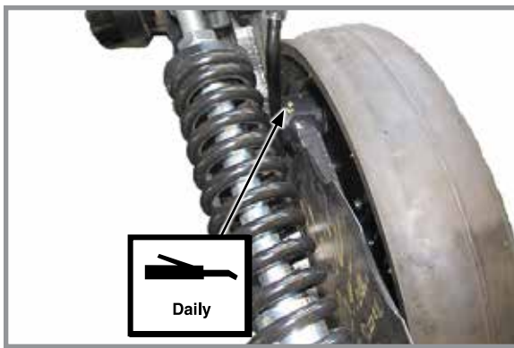
Grease to purge - 1 fitting
