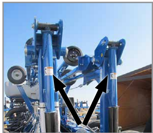
Row Marker Safety Lockup Installed
