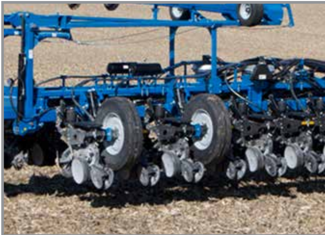
Wing Wheels in Transport Position
