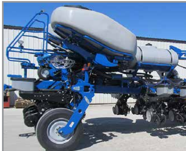
Liquid fertilizer installed on 4900 bulk fill
