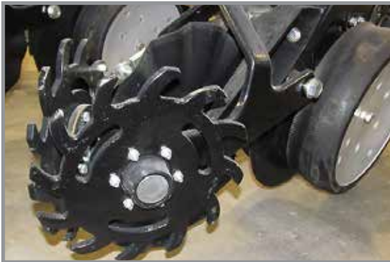
Coulter Mounted Residue Wheels
