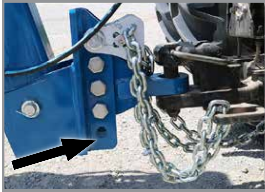
Clevis Adjustment Holes
