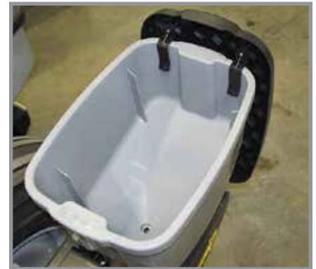
Granular Chemical Hopper
