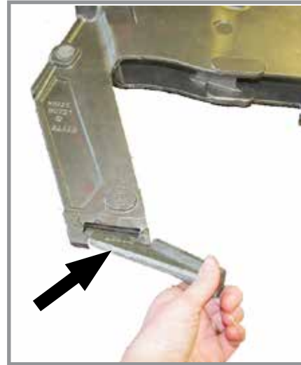
Seed Tube Guard/Inner Scraper (Gauge wheel/seed opener disc blade removed for easier identification of scraper)
