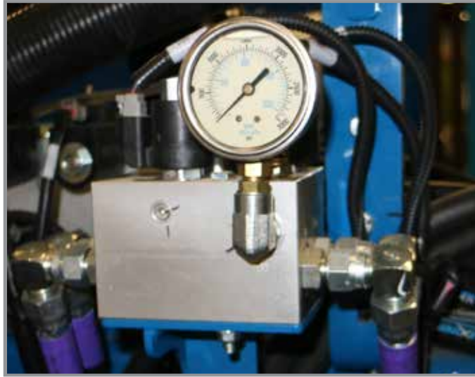
True Depth Pressure Gauge
