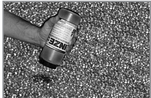
Adding graphite bulk fill hopper
