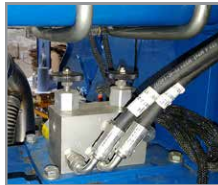
Row Marker Solenoid Valves
