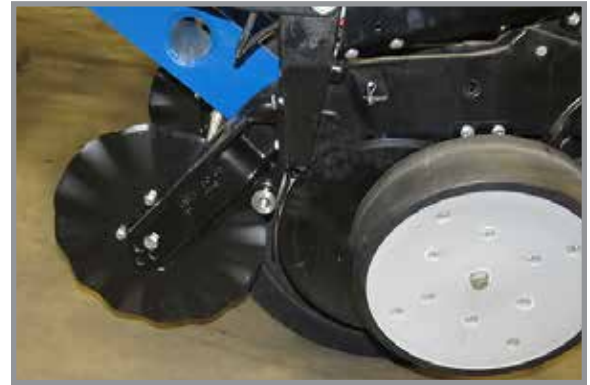
Row Unit Mounted No Till Coulter
