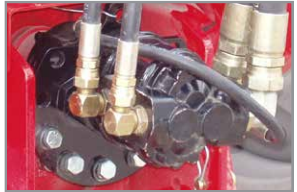
PTO Pump Installed
