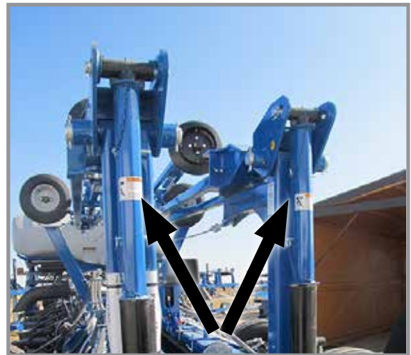
Row Marker Safety Lockup Installed
