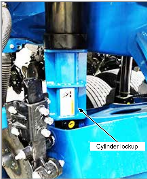
Transport axle cylinder lockup installed
