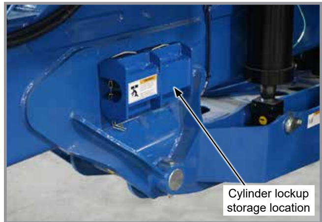
Cylinder lockup storage location
