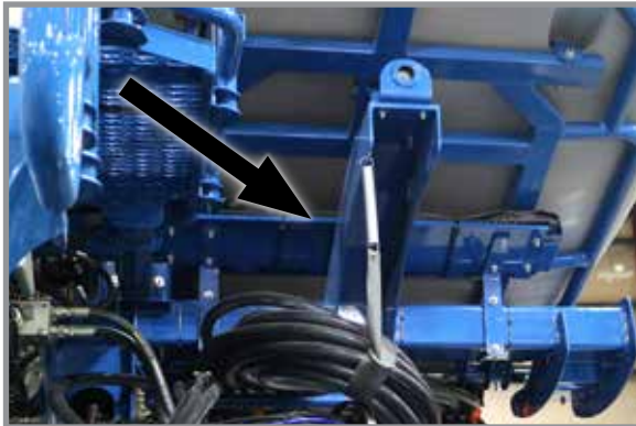
Cleanout Chute Storage Location
