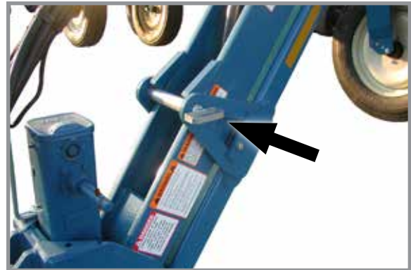
Hitch parallel linkage pin installed
