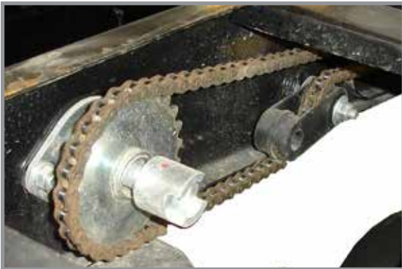
Row unit granular chemical drive
