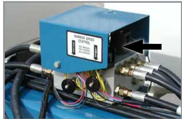
Row marker solenoid valves
