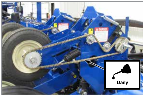
Contact wheel drive chains
