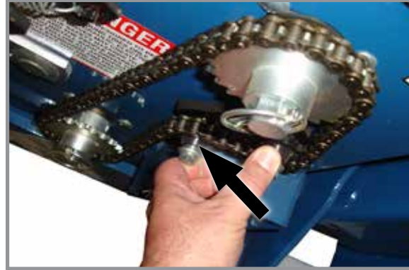
Chain idler tensioning
