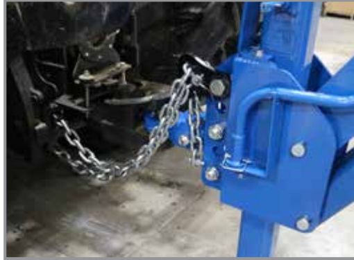
Tractor and safety chain hookup
