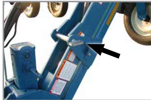
Hitch parallel linkage pin installed
