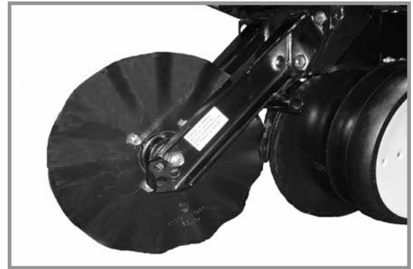
Row unit mounted no till coulter
