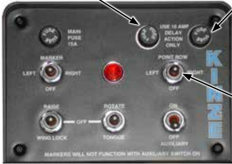
Single point row clutch control box
