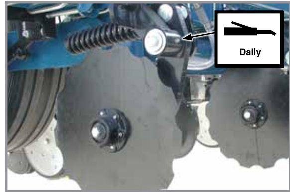
Notched single disc opener (1 per arm)
