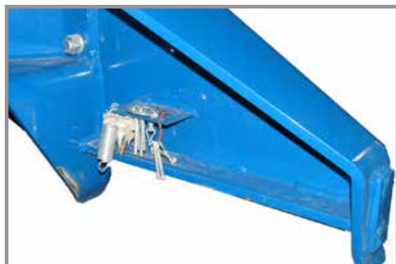
Spare shear pin storage
