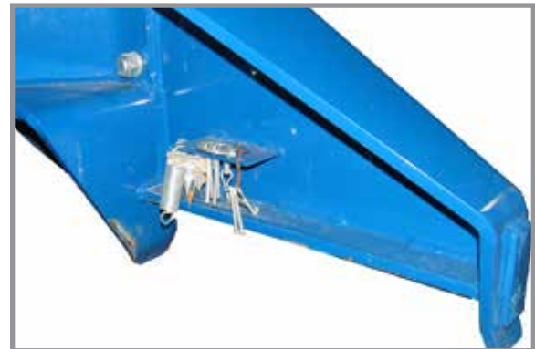
Chain link storage location (each wing)
