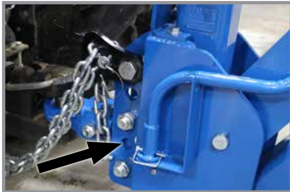
Clevis adjustment holes
