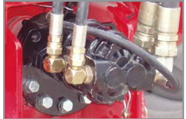
PTO pump installed
