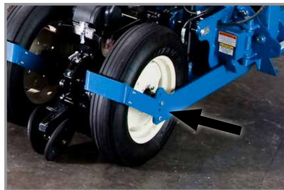
Field/wing wheel adjustment
