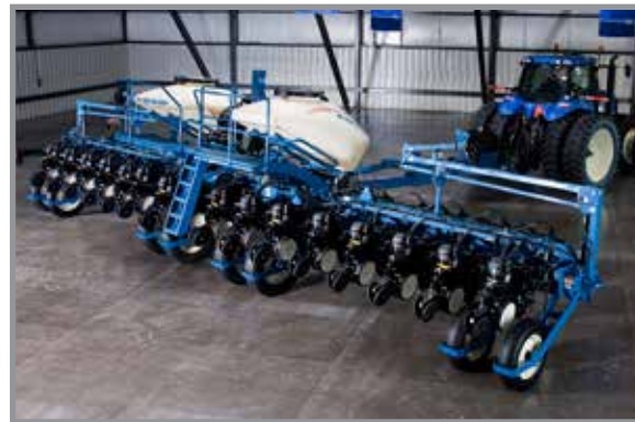
Planter in field lift position
