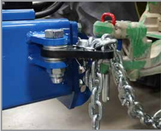
Planter/safety chain hookup to tractor
