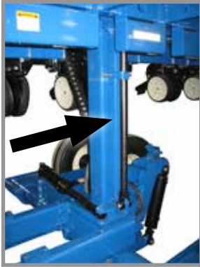
Safety lockup in transport position
