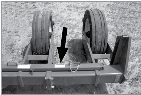
Manual safety lockup in storage position
