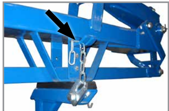
Row marker safety lockup installed
