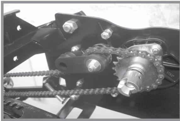
Mechanical push row unit meter drive
