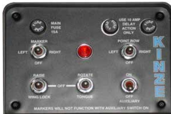
Single point row clutch control box
