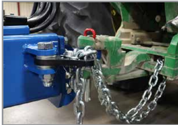
Drawbar and safety chain connection
