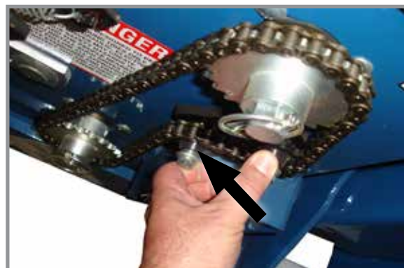
Chain idler tensioning
