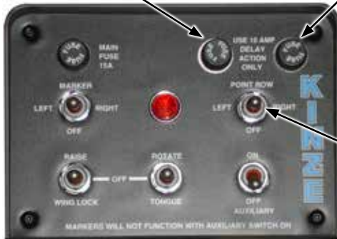
Single point row clutch control box
