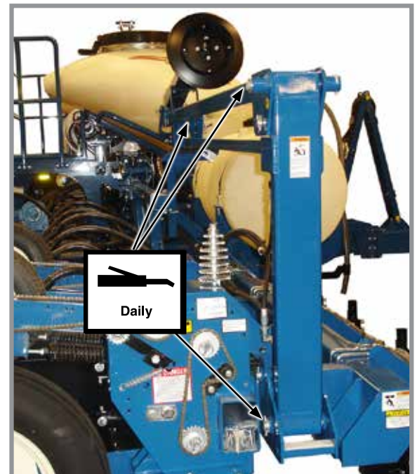
Row marker assemblies - 3 per assembly
