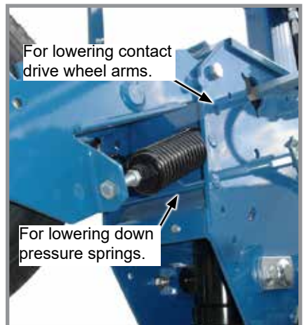
Contact drive wheel adjustment
