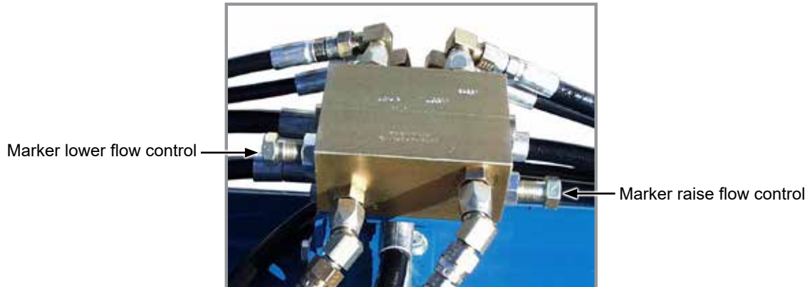
Row marker flow control valves
