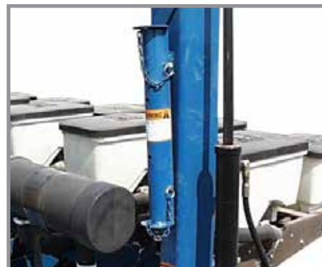
Row marker lockup in storage location
