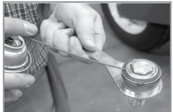
Wrap spring wrench lubrication
