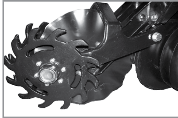
Coulter mounted residue wheels
