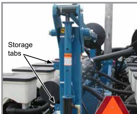
Row marker lockup installed
