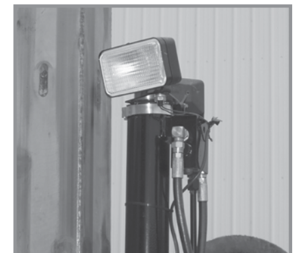
Auxiliary work lights
