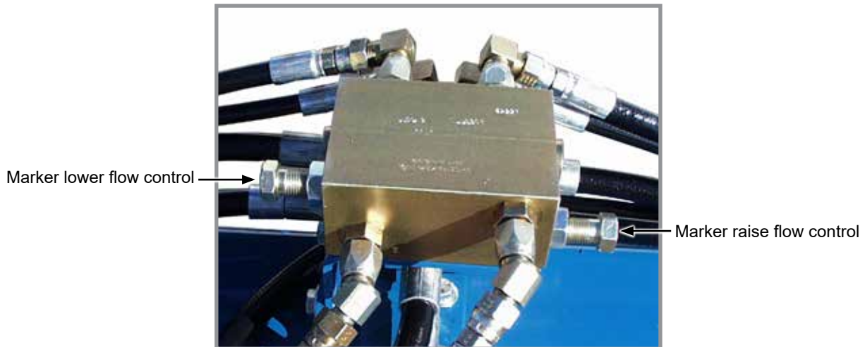
Row marker flow control valves
