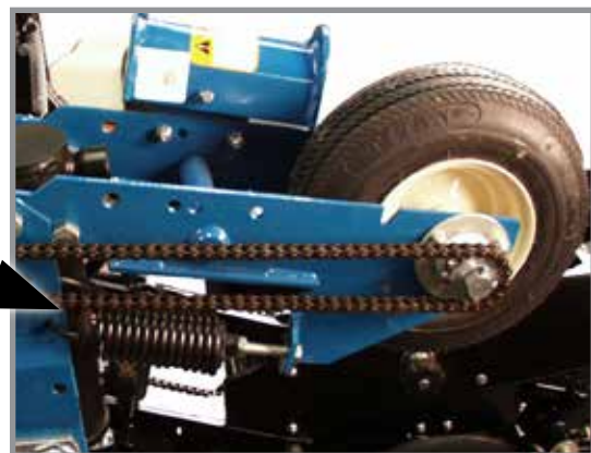
Down pressure spring location
