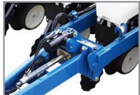
Split Row self-leveling hitch extension
