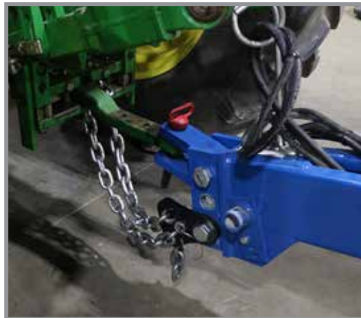
Drawbar and safety chain connection
