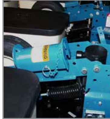
Safety lockup in storage location
