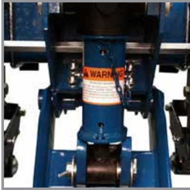
Safety lockup installed
