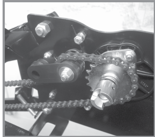
Push row unit meter drive
