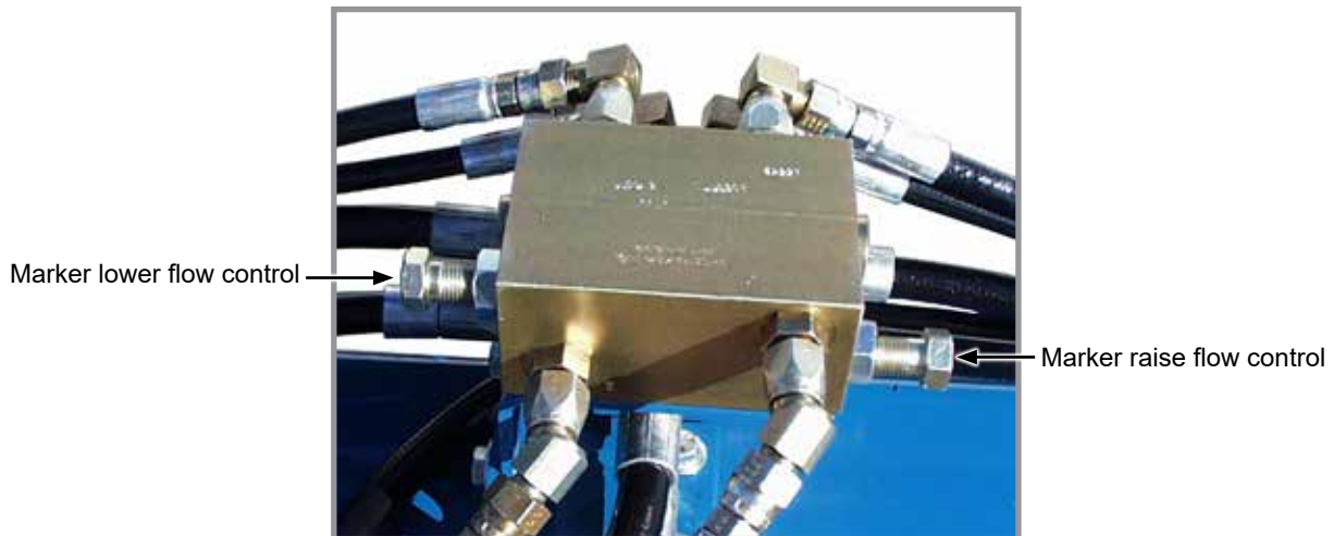
Row marker flow control valves
