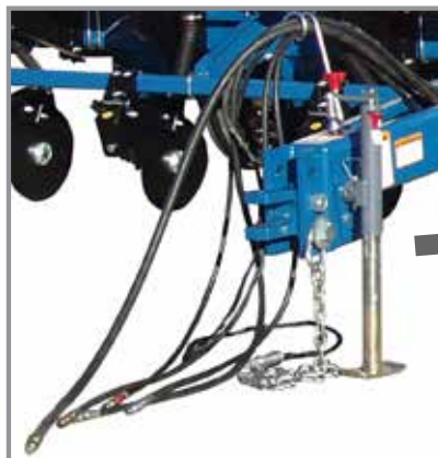
Jack stand installed
