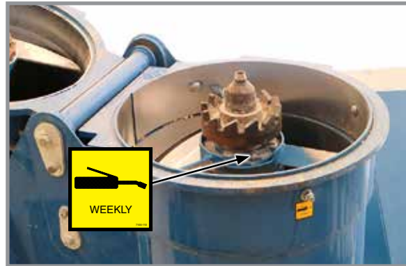
4. Vertical Auger Center Bearing - 1 Zerk (2022 Production)
