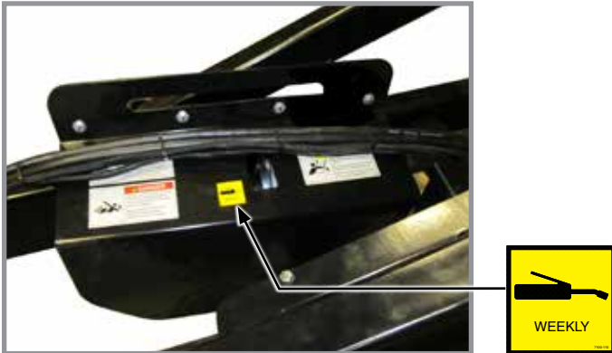
3. Cam Rollers - 1 Zerk (2022 Production)
