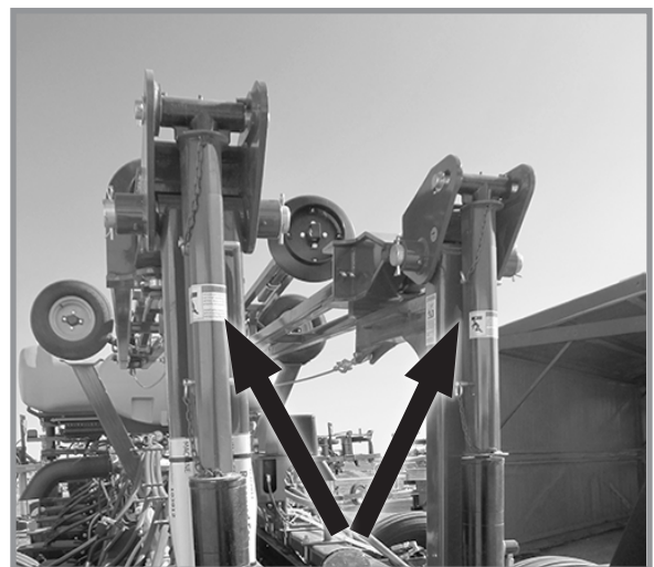
Row Marker Safety Lockup Installed
