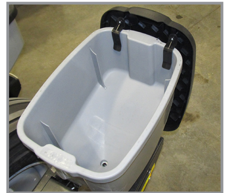
Granular Chemical Hopper
