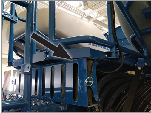
Cleanout Chute Storage Location
