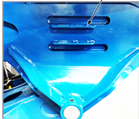
Cylinder lockup storage location
