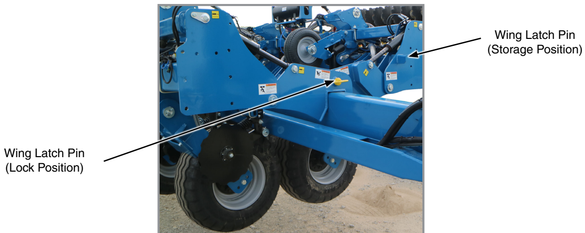
Wing Latch Engaged
