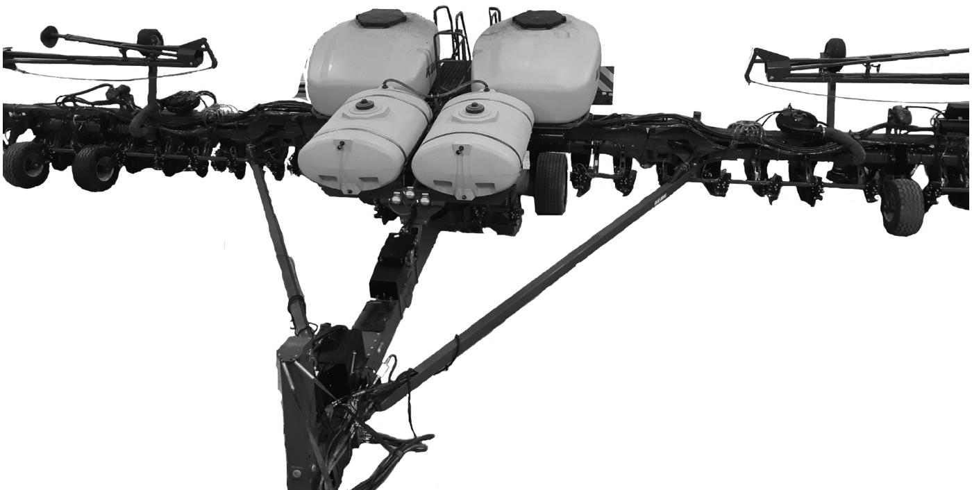
Liquid fertilizer installed on 4800 bulk fill
