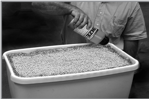
Adding graphite to conventional hopper
