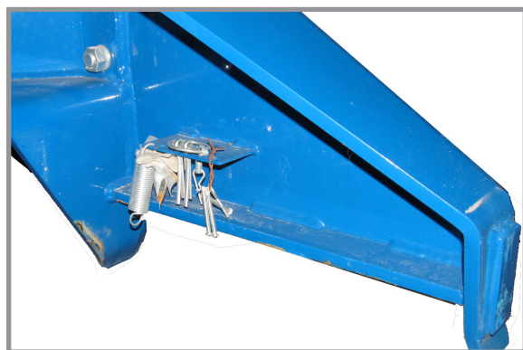
Spare shear pin storage
