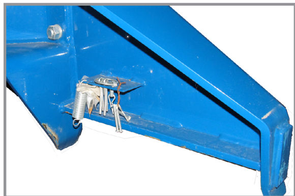
Spare shear pin storage
