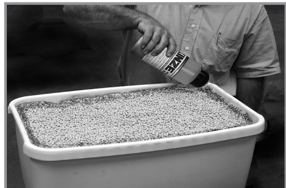
Adding graphite to conventional hopper
