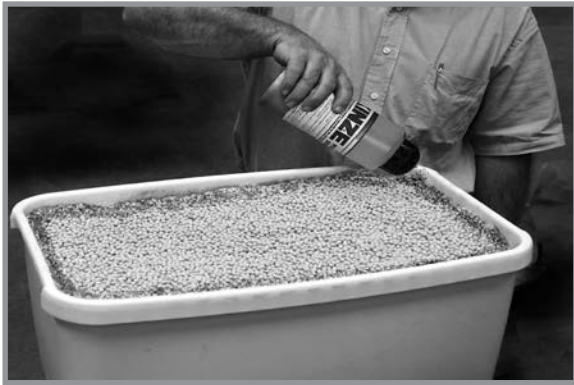
Adding graphite to conventional hopper
