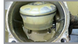
Oil After Diaphragm Rupture
