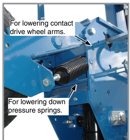
Contact drive wheel adjustment
