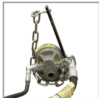
1 \frac{3}{8} "-21 spline PTO pump shown
