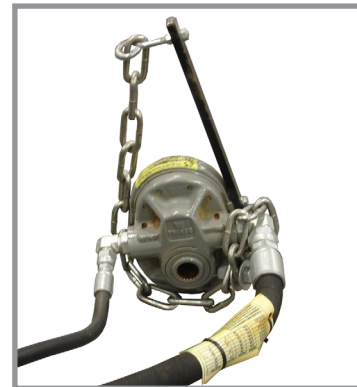
PTO-driven hydraulic pump (1 3/8" spline PTO pump shown)
