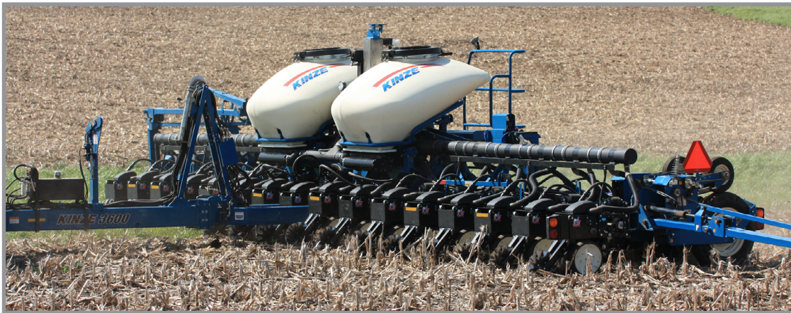
Model 3600 16 Row Planter with Vacuum, Interplant, and Bulk Fill System
