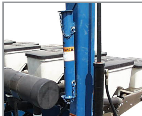
Row marker lockup in storage location
