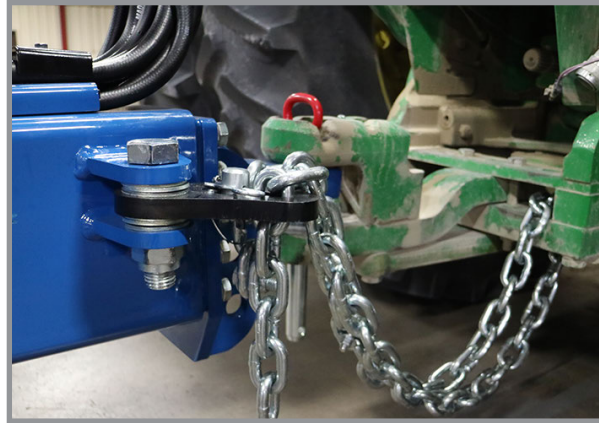
Drawbar and safety chain connection
