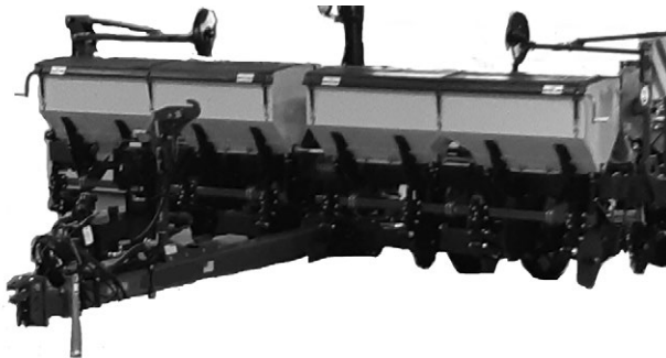
Dry fertilizer option installed
