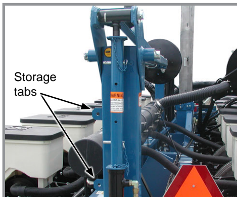
Row marker lockup installed
