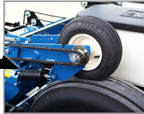
Down pressure spring location
