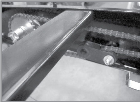
Row unit granular chemical drive
