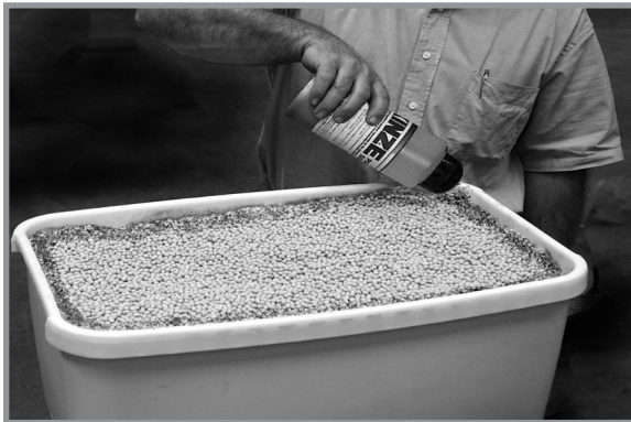
Adding graphite to conventional hopper
