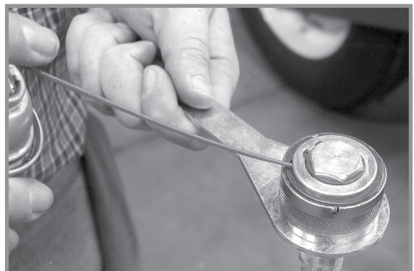
Wrap Spring Wrench Lubrication
