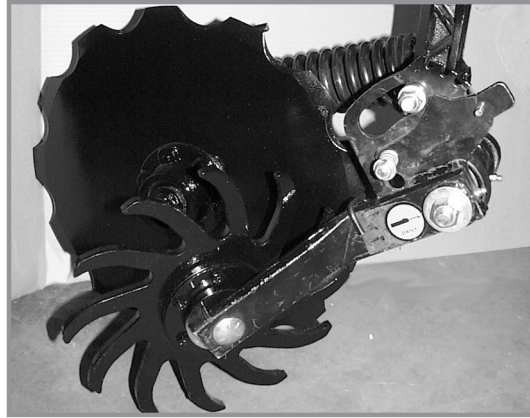
Notched single disc opener residue wheel attachment
