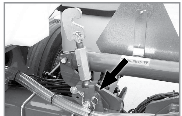
Center turnbuckle lockup pin
