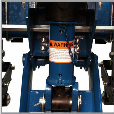
Safety lockup installed
