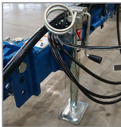
Jack stand installed
