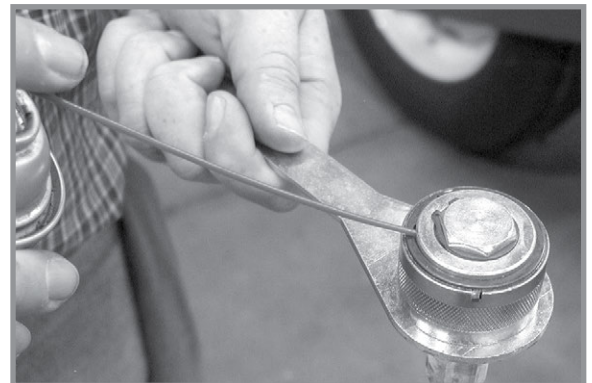
Wrap Spring Wrench Lubrication
