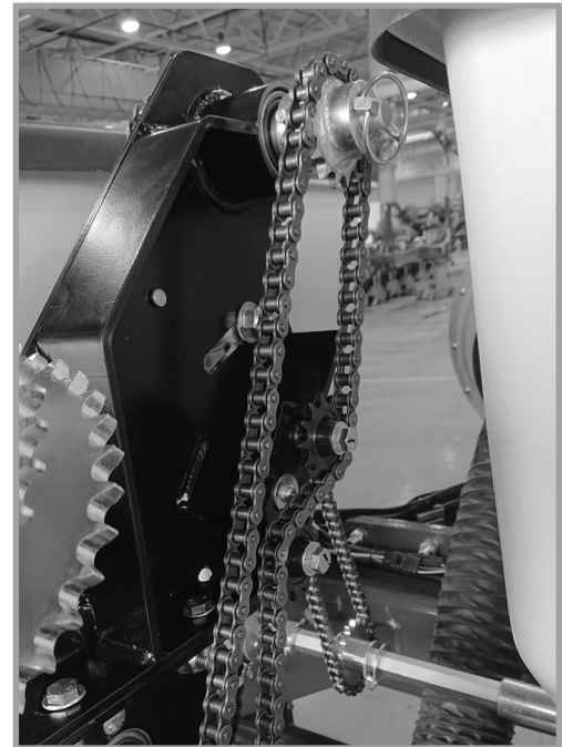
Fertilizer drive rate transmission
