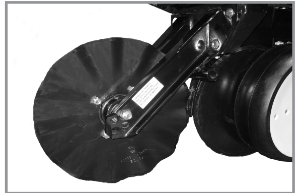
Row unit mounted no till coulters
