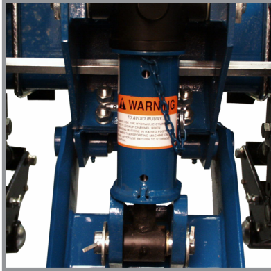
Safety lockup installed
