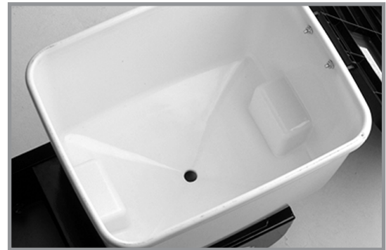
Granular chemical hopper
