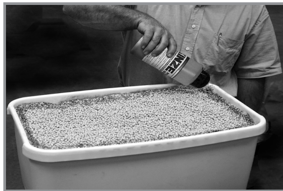
Adding graphite to conventional hopper
