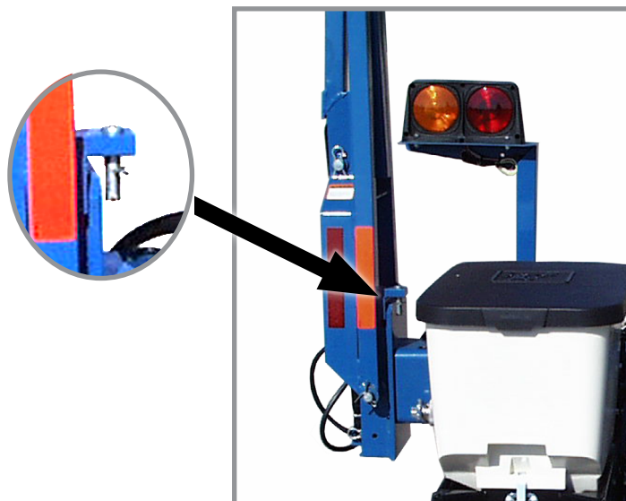
Marker arm safety lockup pin location
