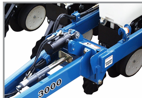
Interplant self-leveling hitch extension
