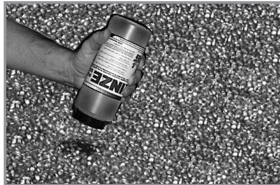
Adding graphite bulk fill hopper
