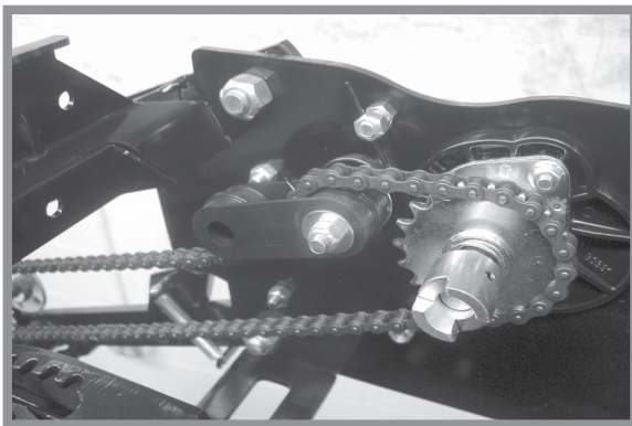
Mechanical push row unit meter drive
