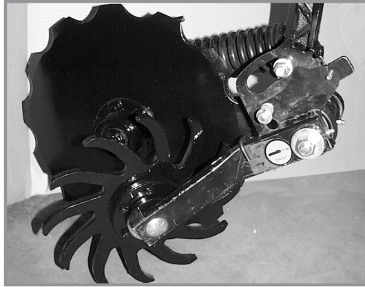
Notched single disc opener residue wheel attachment
