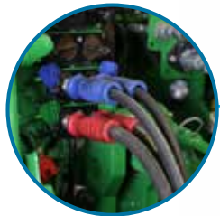
Colored hydraulic handle grips for easy hose identification and hook-ups
