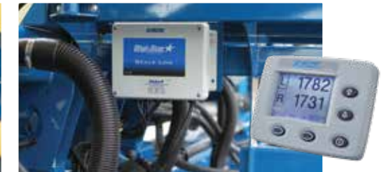
Platform-mounted display installed near hoppers
