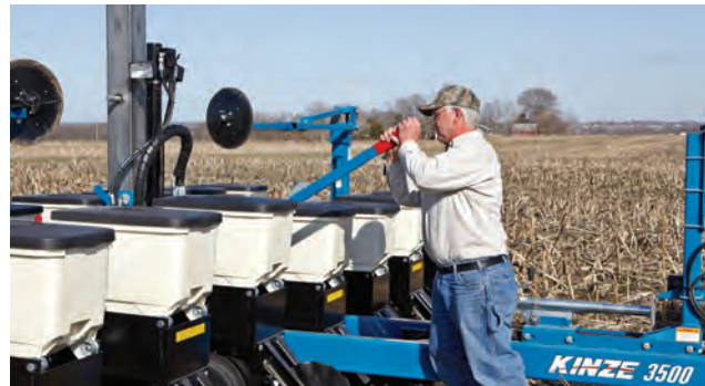
Spring-Loaded Over-Center Row Unit Lock-Ups Easily switch from split rows to standard width rows in minutes.
