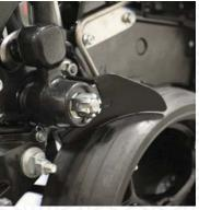
Spoked gauge wheels equipped with heavy-duty, long-life steel scrapers
